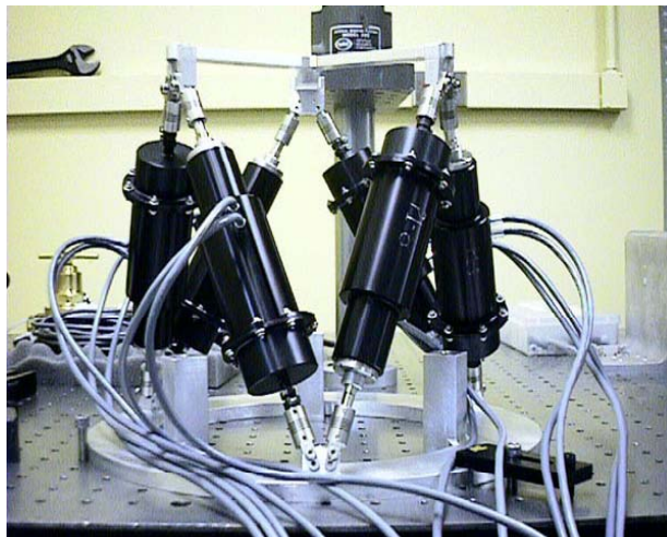
Figure 7: Developmental Comparative Active Telescope Testbed with Inchworm actuators - NASA
