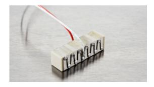
Noliac plate stack actuator NAC2003-Hxx (height in mm – Hxx) is based on the multilayer actuator NAC2003 and can be stacked to match you requirements. The standard range of NAC2003-Hxx is produced in a height between 4-50 mm. The plate stack provides a stroke up to 72  $\mu$ m and blocking force up to 1050 N depending on the height of the stack.
