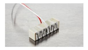
Noliac plate stack actuator NAC2012-Hxx (height in mm – Hxx) is based on the multilayer actuator NAC2012 and can be stacked to match your requirements. The standard range of NAC2012-Hxx is produced in a height between 4-30 mm. The plate stack provides a stroke up to 43.89  $\mu m$  and blocking force up to 378 N depending on the height of the stack.
