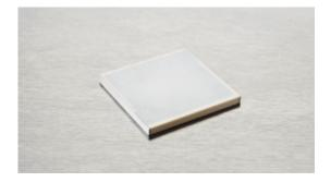
The multilayer piezo actuators can reach full performance at very low operating voltage. The plate actuator NAC2021 is 7x7 mm and provides a free stroke of 3.3  $\mu$ m and a blocking force of 2060 N.
