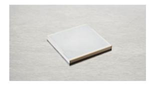
The multilayer piezo actuators can reach full performance at very low operating voltage. The plate actuator NAC2022 is 10x10 mm and provides a free stroke of 3.3  $\mu$ m and a blocking force of 4200 N.
