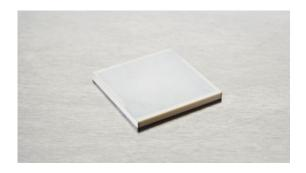
The multilayer piezo actuators can reach full performance at very low operating voltage. The plate actuator NAC2023 is 15x15 mm and provides a free stroke of 3.3  $\mu$ m and a blocking force of 9450 N.
