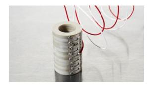
Noliac ring stack actuator NAC2124-Hxx (height in mm – Hxx) is based on the multilayer actuator NAC2124 and can be stacked to match you requirements. The standard range of NAC2124-Hxx is produced in a height between 4-150 mm. The ring stack provides a stroke in a range between 3.3 and 244.2  $\mu$ m and blocking force up to 4750 N depending on the height of the stack.
