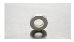
The Noliac piezo actuators can reach full performance at very low operating voltage. The ring actuator NAC2124 is 15x9 mm with a free stroke of 3.3  $\mu$ m and a blocking force of 4750 N.
