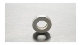
The Noliac piezo actuators can reach full performance at very low operating voltage. The ring actuator NAC2125 is 20x12 mm with a free stroke of 3.3  $\mu$ m and a blocking force of 8450 N.
