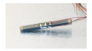
The NAC2910 offers double s-movement and is available as a prototype. Note that the NAC2910 moves with a parallel level at the top. The bender measures 28x2.5x2.5 mm and provides a stroke of +/- 35  $\mu$ m and a blocking force of 3.8 N.
