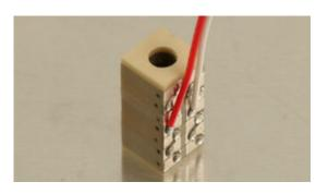
Noliac piezo actuators can be produced with a through hole. This feature is widely used in optical applications, where the inner hole serves as a clear aperture for light beams or optical fibers. The through hole can also be used for applying preload, or for instance to install measuring equipment in the axis of the stack.
