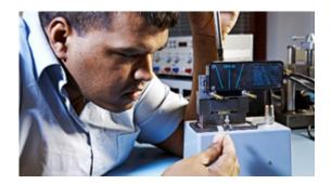
For a number of applications it is necessary to test the piezo components in harsh conditions or with a realistic load. We can also increase the confidence level (100% vs. AQL). For industries like space and medical, there are regulations that implies additional testing. To be able to investigate individual elements, we also offer traceability.
