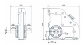
The output shaft and mounting bracket can be adapted to your specific needs. The PAD can be adapted for front/rear mounting, and the shaft can be cross drilled, slotted, hollow etc. Contact us with your specific interface.
