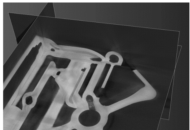
Figure 8. Three-axis view of CT scan of AM valve body
