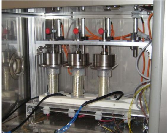
**Fig. 7:** Prototype LV DEAPs on test bench in climate chamber.
