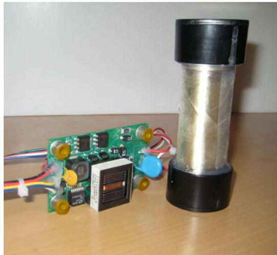
**Fig. 1:** Comparison of a DEAP actuator and an adapted commercial driving unit (courtesy of Danfoss Polypower).
