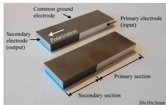
Fig. 1: IDE piezoelectric transformer.
