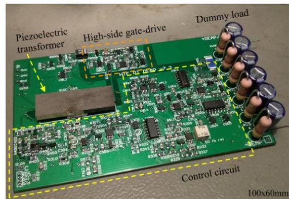
**Fig. 3:** The bi-directional PT based prototype driver, illustrating the general circuit layout.
