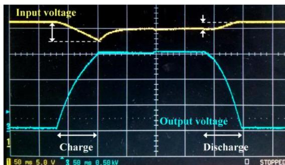
**Fig. 4:** Input and output voltage waveforms, demonstrating driver functionality.
