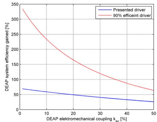
**Fig. 9:** DEAP system efficiency gain when utilizing a bi-directional driver.
