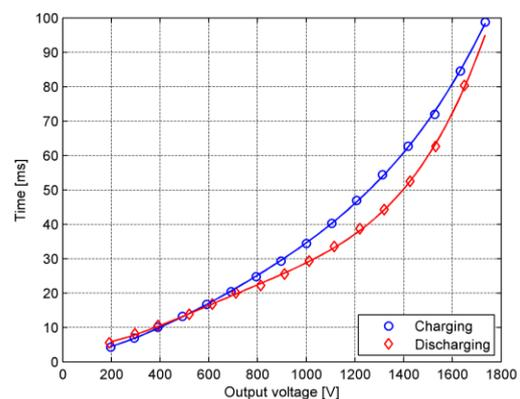
**Fig. 7:** Charge and discharge time of 100nF load.
