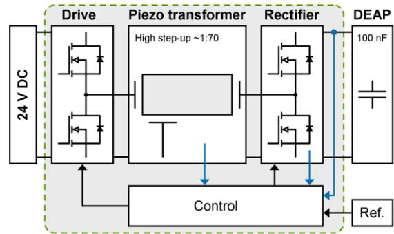
**Fig. 2:** Block diagram of the bi-directional PT topology.
