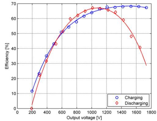
**Fig. 5:** Driver efficiency of a full charging and full discharging period.
