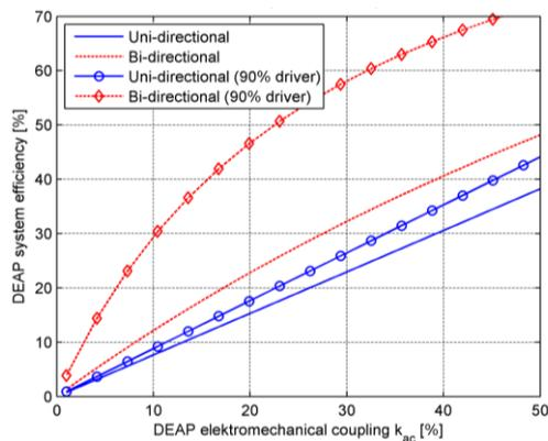
**Fig. 8:** DEAP system efficiency with the presented driver efficiencies and a 90% efficient driver.
