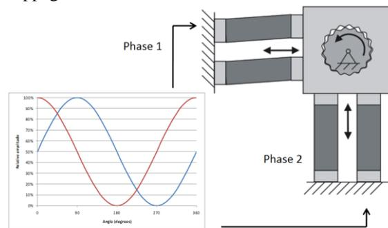
**Fig. 1:** Basic principle of PAD motor
