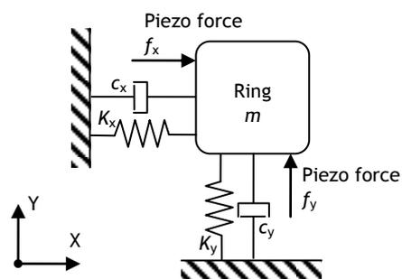
**Fig. 5: Dynamic model of the stator**
