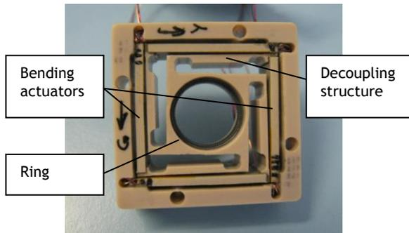
**Fig. 2: PAD motor stator**
