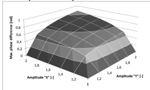
**Fig. 4: Maximum allowable phase error**
