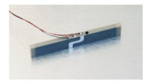
The NAC2810 offers single s-movement and is available as a prototype. The main feature of this product is that it is much stiffer in the direction of action than in the perpendicular direction. The bender measures 40x8x2 mm and provides a stroke of  $\pm$ 1- 34  $\pm$ 2 mm and a blocking force of 0.27 N.
