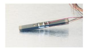
The NAC2910 offers double s-movement and is available as a prototype. Note that the NAC2910 moves with a parallel level at the top. The bender measures 28x2.5x2.5 mm and provides a stroke of +/- 35  $\mu$ m and a blocking force of 3.8 N.
