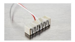
Parallelism ensures optimal performance of your piezo actuator stacks. Noliac offers parallelism with high accuracy for stacks with cross sections of 5x5 mm, 7x7 mm and 10x10 mm and a variety of lengths. 10x10 mm stacks have a plane parallelism of  $<10\mu$ m, and 7x7 mm stacks have a plane parallelism of  $<5\mu$ m.
