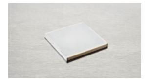
The Noliac multilayer piezo actuators can reach full performance at very low operating voltage. The plate actuator NAC2001 is the smallest of our standard plate actuators ranging only 2x2 mm with a free stroke of 3  $\mu$ m and a blocking force of 168 N.
