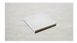
The multilayer piezo actuators can reach full performance at very low operating voltage. The plate actuator NAC2011 is 2x2 mm and provides a free stroke of 3.3  $\mu$ m and a blocking force of 168 N.
