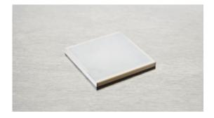
The multilayer piezo actuators can reach full performance at very low operating voltage. The plate actuator NAC2013 is 5x5 mm and provides a free stroke of  $3.3 \mu$ m and a blocking force of 1050 N.
