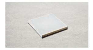
The multilayer piezo actuators can reach full performance at very low operating voltage. The plate actuator NAC2014 is 7x7 mm and provides a free stroke of 3.3  $\mu$ m and a blocking force of 2060 N.
