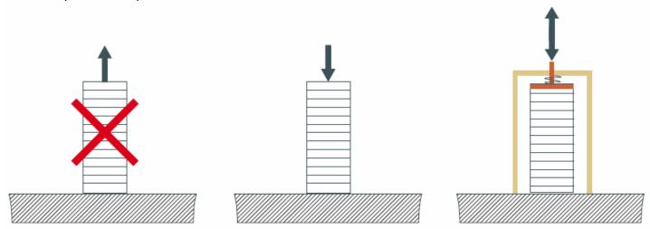
For linear actuators it is recommended not to use a metal plate on top and bottom in order to avoid short circuit.
