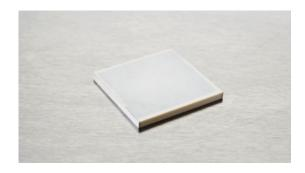
The multilayer piezo actuators can reach full performance at very low operating voltage. The plate actuator NAC2025 is 5x5 mm and provides a free stroke of 1.9  $\mu$ m and a blocking force of 800 N.
