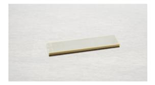
Noliac plate benders are manufactured with ceramic layer thickness down to  $67\mu$ m as standard to facilitate very low operating voltage for full performance of the piezo material. CMBP02 measures 21x7.8x1.3 mm. The plate bender provides stroke of +/- 120  $\mu$ m and a blocking force of 3.7 N.
