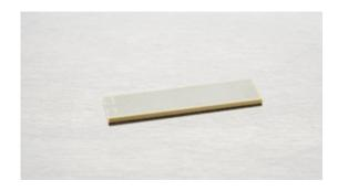
Noliac plate benders are manufactured with ceramic layer thickness down to  $67\mu m$  as standard to facilitate very low operating voltage for full performance of the piezo material. CMBP05 measures 32x7.8x1.3 mm. The plate bender provides stroke of  $\pm 1.345$   $\mu m$  and a blocking force of 2.25 N.
