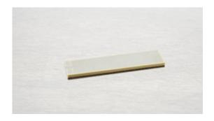
Noliac plate benders are manufactured with ceramic layer thickness down to  $67\mu m$  as standard to facilitate very low operating voltage for full performance of the piezo material. CMBP07 measures 50x7.8x0.7 mm. The plate bender provides stroke of +/-  $1270~\mu m$  and a blocking force of 0.4~N.
