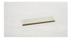
Noliac plate benders are manufactured with ceramic layer thickness down to  $67\mu$ m as standard to facilitate very low operating voltage for full performance of the piezo material. CMBP08 measures 50x7.8x1.3 mm. The plate bender provides a stroke of +/- 850 µm and a blocking force of 1.6 N.
