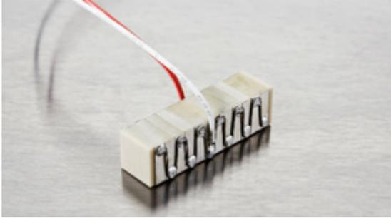
Noliac plate stack actuator NAC2001-Hxx (height in mm – Hxx) is based on the multilayer actuator NAC2001 and can be stacked to match your requirements. The standard range of NAC2001-Hxx is produced in a height between 4-20 mm. The plate stack provides a stroke up to 22.9  $\mu\text{m}$  and blocking force up to 168 N depending on the height of the stack.
