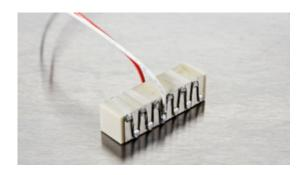
oliac plate stack actuator NAC2002-Hxx (height in mm – Hxx) is based on the multilayer actuator NAC2002 and can be stacked to match you requirements. The standard range of NAC2002-Hxx is produced in a height between 4-30 mm. The plate stack provides a stroke up to 39.9  $\mu m$  and blocking force up to 378 N depending on the height of the stack.
