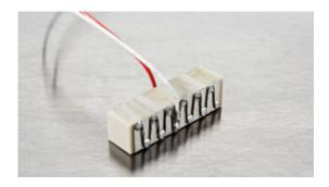
Noliac plate stack actuator NAC2013-Hxx (height in mm – Hxx) is based on the multilayer actuator NAC2013 and can be stacked to match you requirements. The standard range of NAC2013-Hxx is produced in a height between 4-50 mm. The plate stack provides a stroke up to 79.2 µm and blocking force up to 1050 N depending on the height of the stack.
