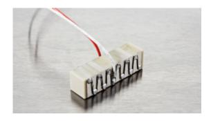
Noliac plate stack actuator NAC2022-Hxx (height in mm – Hxx) is based on the multilayer actuator NAC2022 and can be stacked to match you requirements. The standard range of NAC2022-Hxx is produced in a height between 4-100 mm. The plate stack provides a stroke up to 161.7  $\mu m$  and blocking force up to 4200 N depending on the height of the stack.
