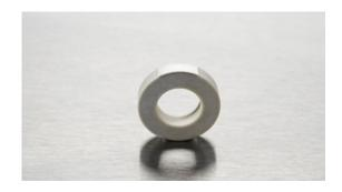
The Noliac piezo actuators can reach full performance at very low operating voltage. The ring actuator NAC2122 is 8x3 mm and provides a free stroke of 3.3  $\mu$ m and a blocking force of 1810 N.
