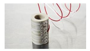
Noliac ring stack actuator NAC2121-Hxx (height in mm – Hxx) is based on the multilayer actuator NAC2121 and can be stacked to match you requirements. The standard range of NAC2121-Hxx is produced in a height between 4-60 mm. The ring stack provides a stroke in a range between 3.3 and 95.7 µm and blocking force up to 1060 N depending on the height of the stack.
