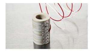
Noliac ring stack actuator NAC2122-Hxx (height in mm – Hxx) is based on the multilayer actuator NAC2122 and can be stacked to match you requirements. The standard range of NAC2122-Hxx is produced in a height between 4-80 mm. The ring stack provides a stroke in a range between 3.3 and 128.7  $\mu$ m and blocking force up to 1810 N depending on the height of the stack.
