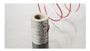
Noliac ring stack actuator NAC2123-Hxx (height in mm – Hxx) is based on the multilayer actuator NAC2123 and can be stacked to match you requirements. The standard range of NAC2123-Hxx is produced in a height between 4-120 mm. The ring stack provides a stroke in a range between 3.3 and 194.7  $\mu$ m and blocking force up to 3560 N depending on the height of the stack.
