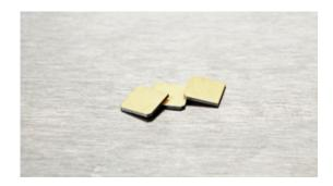
The Noliac shear plate actuators are characterized by providing a large stroke for a very compact design. The shear plate CSAP01 measures 2x2x0.5 mm and provides a free stroke of  $1.5~\mu m$  and a capacitance of 133~pF.
