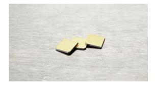
The Noliac shear plate actuators are characterized by providing a large stroke for a very compact design. The shear plate CSAP02 measures 5x5x0.5 mm and provides a free stroke of 1.5 µm and a capacitance of 830 pF.
