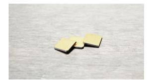
The Noliac shear plate actuators are characterized by providing a large stroke for a very compact design. The shear plate CSAP03 measures 10x10x0.5 mm and provides a free stroke of 1.5 µm and a capacitance of 3.321 pF.
