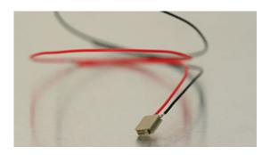
The Noliac shear stack NAC2403-H1.7 features shear motion on the X-axis. This product is ideal for stick-slip and nanopositioning applications. NAC2403-H1.7 measures 10x10 mm with a height of 1.7 mm and provides free stroke of 1.5  $\mu$ m and a capacitance of 3.3 nF. End plates on top and bottom are included. The shear stack has ultra thin electrodes made of standard steel as standard.
