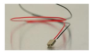
The Noliac shear stack NAC2403-H2.3 features shear motion on the X-axis. This product is ideal for stick-slip and nanopositioning applications. NAC2403-H2.3 measures 10x10 mm with a height of 2.3 mm and provides a free stroke of 3  $\mu$ m and a capacitance of 6.6 nF. End plates on top and bottom are included. The shear stack has ultra thin electrodes made of standard steel as standard.
