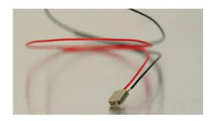
The Noliac shear stack NAC2902-H2.8 features shear motion on the X/Y-axis. This product is ideal for stick-slip and nanopositioning applications. NAC2902-H2.8 measures 5x5 mm with a height of 2.8 mm and provides free stroke of 1.5/1.5  $\mu$ m and a capacitance of 0.8/0.8 nF. End plates on top and bottom are included. The shear stack has ultra thin electrodes made of standard steel as standard.
