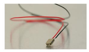
The Noliac shear stack NAC2902-H4 features shear motion on the X/Y-axis. This product is ideal for stick-slip and nanopositioning applications. NAC2902-H4 measures 5x5 mm with a height of 4 mm and provides a free stroke of 3/3  $\mu$ m and a capacitance of 1.7/1.7 nF. End plates on top and bottom are included. The shear stack has ultra thin electrodes made of standard steel as standard.
