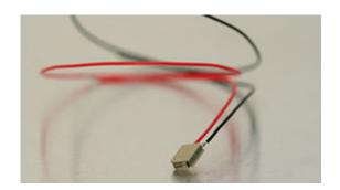
The Noliac shear stack NAC2903-H2.8 features shear motion on the X/Y-axis. This product is ideal for stick-slip and nanopositioning applications. NAC2903-H2.8 measures 10x10 mm with a height of 2.8 mm and provides a free stroke of 1.5/1.5  $\mu$ m and a capacitance of 3.3/3.3 nF. End plates on top and bottom are included. The shear stack has ultra thin electrodes made of standard steel as standard.
