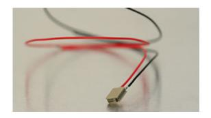
The Noliac shear stack NAC2903-H4 features shear motion on the X/Y-axis. This product is ideal for stick-slip and nanopositioning applications. NAC2903-H4 measures 10x10 mm with a height of 4 mm and provides free stroke of 3/3  $\mu$ m and a capacitance of 6.6/6.6 nF. End plates on top and bottom are included. The shear stack has ultra thin electrodes made of standard steel as standard.
