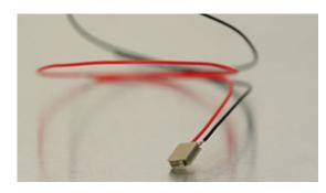
The Noliac shear stack NAC2903-H6.4 features shear motion on the X/Y-axis. This product is ideal for stick-slip and nanopositioning applications. NAC2903-H6.4 measures 10x10 mm with a height of 6.4 mm and provides free stroke of 6/6  $\mu$ m and a capacitance of 13.3/13.3 nF. End plates on top and bottom are included. The shear stack has ultra thin electrodes made of standard steel as standard.
