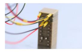
The Noliac shear stack NAC3402-H12.6 features motion in the X/Y/Z-axis. This product is ideal for stick-slip and nanopositioning applications. NAC3402-H12.6 measures 5x5 mm with a height of 12.6 mm and provides free stroke of 3/3/3  $\mu$ m and a capacitance of 1.7/1.7/11.1 nF. End plates on top and bottom are included. The shear stack has ultra thin electrodes made of standard steel as standard.
