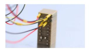
The Noliac shear stack NAC3403-H7.4 features motion in the X/Y/Z-axis. This product is ideal for stick-slip and nanopositioning applications. NAC3403-H7.4 measures 10x10 mm with a height of 7.4 mm and provides free stroke of 1.5/1.5/1.5 µm and a capacitance of 3.3/3.3/21.4 nF. End plates on top and bottom are included. The shear stack has ultra thin electrodes made of standard steel as standard.
